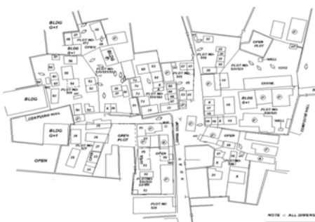
Re-done Plane Table Survey by SPARC-UDRC -OSDF-MM, 2010
